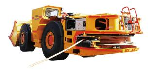
FL14E is an electric LHD designed for large scale underground metal mines production, payload 14 mt.
