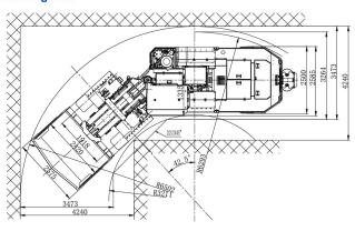
FL14 is a diesel engine LHD designed for large scale underground metal mines production, payload 14 mt
