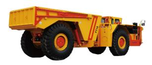
FT15 is a 15 ton payload, front-facing operated mining truck for underground long distance ore transportation. It has compact design, small turning radius, and big dumping angle. It applies Volvo TAD850VE 160 Kw Engine and other brands component, to meet tough UG road conditions.
